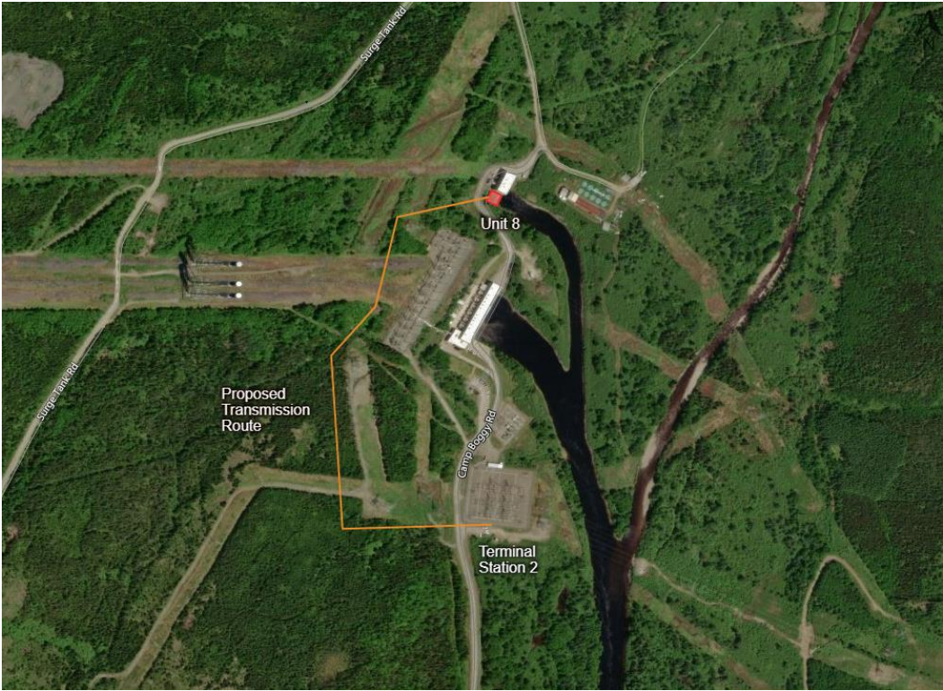
Figure 4: Transmission Line Route
